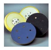
The low profile design (1/2" thick) is specifically balanced to eliminate vibration to enhance fine grit sanding. Designed with medium density polyurethane foam for conformability, these pads are firm enough for flat surfaces. The vacuum is available in standard 5-hole pattern or a 6-hole pattern. The backing plate is fiberglass with a riveted 5/16"-24 threaded shank.
