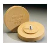
This wheel is designed to remove pinstripes, decals and molding adhesive without damage to the underlying surface. Tan colored, it is 4" diameter, 5/8" thick with a 1/16" step and has a 5/16-24 attached threaded mandrel.
