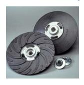
For fibre discs and Bear-Tex abrasive brushes, these pads are designed for medium to heavy grinding applications. Slotted aluminum hub plus curved ribs on rubber face of pad promote a cooler cutting action to reduce loading and increase abrasive life by up to 20%. Fits 5/8"-11 arbor. Choose medium density for all-purpose grinding; hard density for a more aggressive cut. Select retainer nut for pad of your choice.
