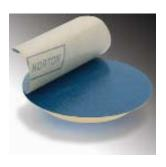
Designed for use with all PSA (pressure sensitive adhesive) backed discs. Made of epoxyglass and molded rubber, the 6" pads (3/4" thick) have a 5/16"-24 threaded shank for use on random orbital or dual action sanders. The 8" pad has a 5/8"-11 threaded female hub.
